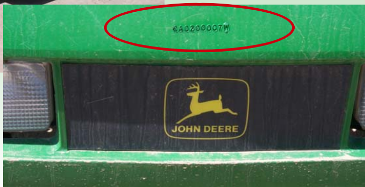
Right : Owner Applied Number (OAN) stamped on to the front of the John Deere Gator
